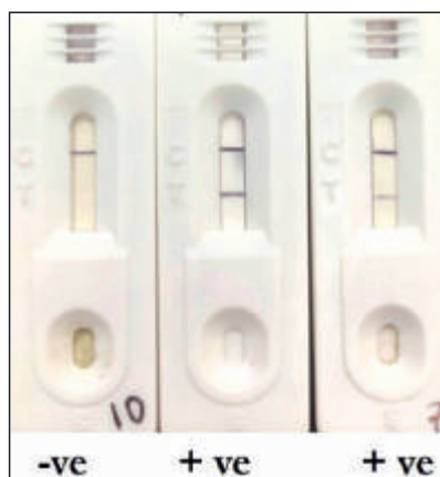
Figure 21: LFA kit developed for the detection of Nosema infection in silkworms. Colour development was seen both in negative samples (single band) and Nosema infected positive samples (two bands).
